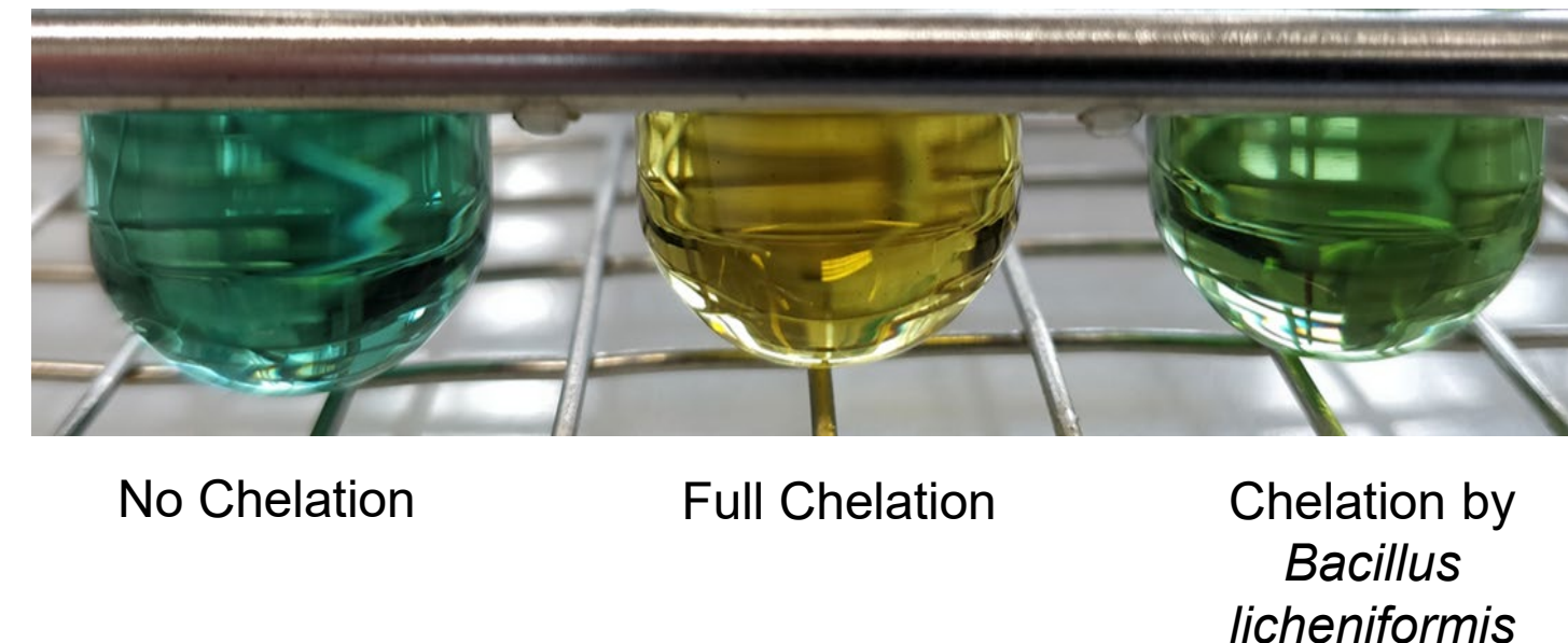
Fig. 2. Siderophore detection in Bacillus licheniformis G3 (ATCC PTA-127113) by iron chelation using CAS assay
